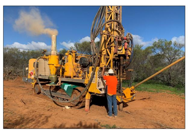
Fig. 1- Santy Project, aircore drilling underway at the Coastal target.
